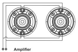
Series-Parallel 2x Dual 4 ohm sub = 4 ohm
