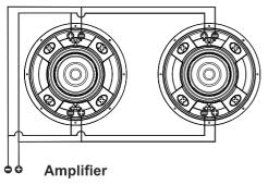
Parallel-Parallel 2x Dual 4 ohm subs = 1 ohm
